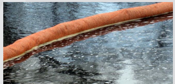
Product no. 77608 Absorption boom 25 meter x Ø15 cm (can absorb up to 440 litres oil – chemicals)
